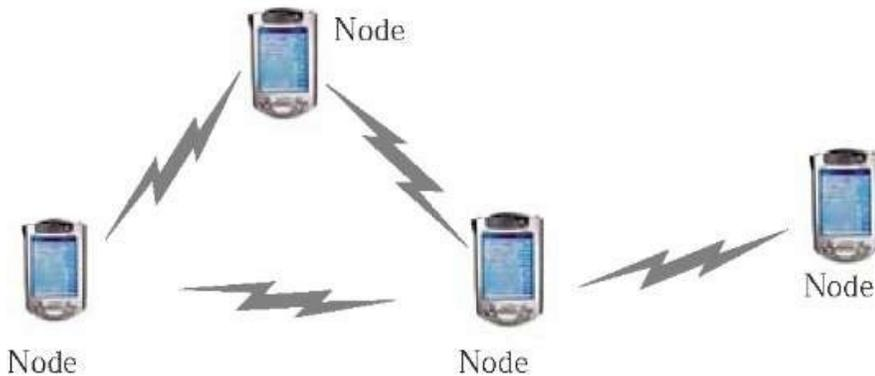
The way that this network will operate is by using the DSR protocol. DSR is intended to be used with mesh networks and works by building routing tables at each node. In this way, nodes will know the path to send a packet rather than determining the next step at each node. Additionally, the encryption will be based on the public key methods that are commonly used today.
